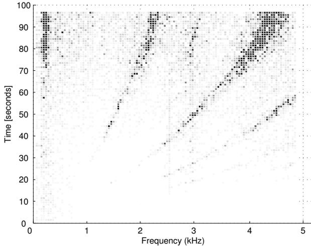
**Figure 3. Helicopter sound spectrum in transition from 0% to 100% motor power.**
