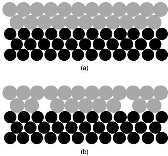
FIG. 6. Interfaces in a compressive strained-layer system: (a) coherent; (b) decorated with vacancies.
