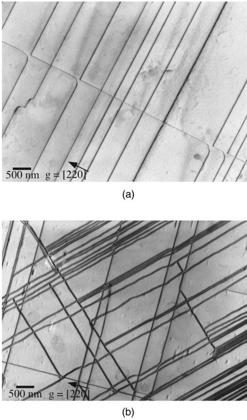
FIG. 4. Misfit dislocations in GaAs/In<sub>0.2</sub>Ga<sub>0.8</sub>As (20 nm)/GaAs: (a) 60° dislocations in the as-grown specimen, (b) after thermal processing at 1040 K.
