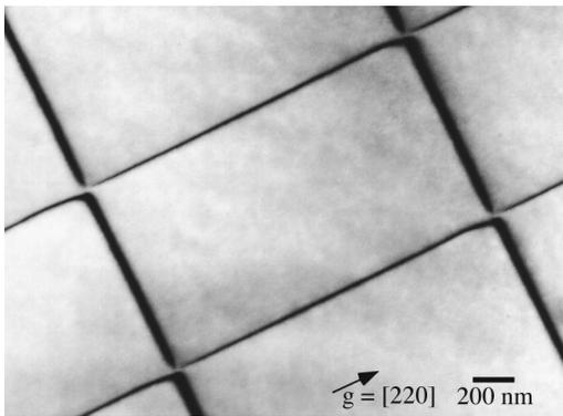
FIG. 2. 60° misfit dislocations in as-grown GaAs/In<sub>0.15</sub>Ga<sub>0.85</sub>As (25 nm)/GaAs (TEM bright field image).
