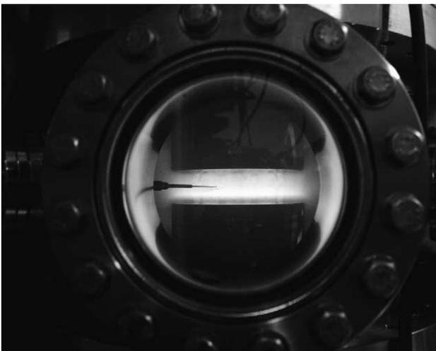
Fig. 2. Langmuir probe inserted into an Argon plasma.
