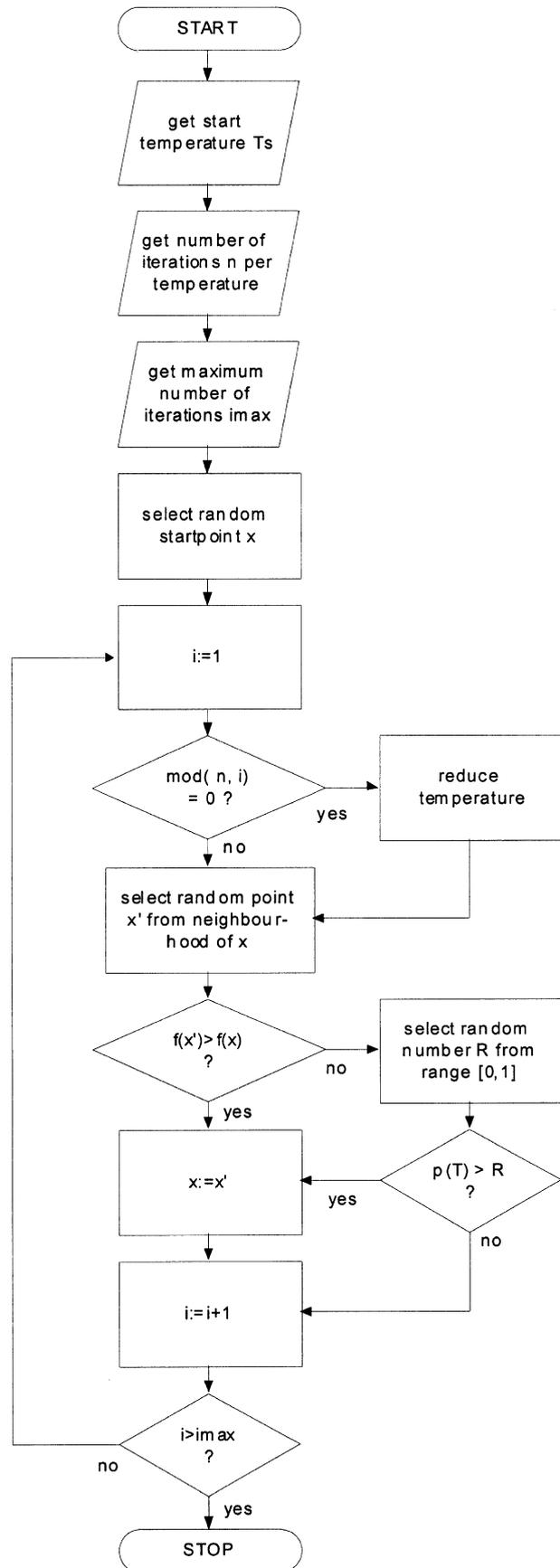
Fig. 4. Flow-chart of the basic SA algorithm.
