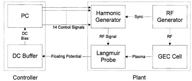
Fig. 3. Closed control loop for waveform tuning.
