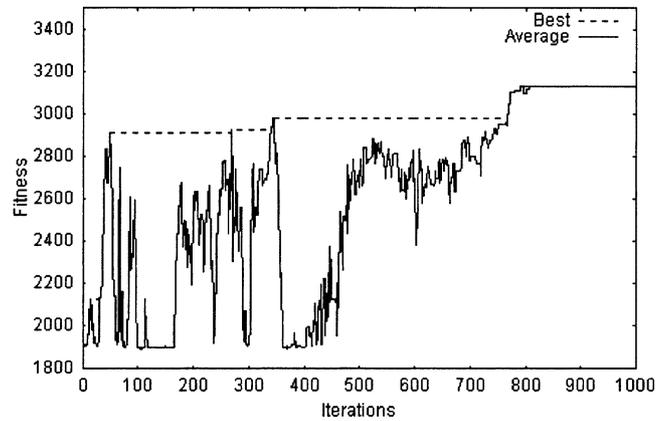
Fig. 9. Typical run of the SA algorithm.
