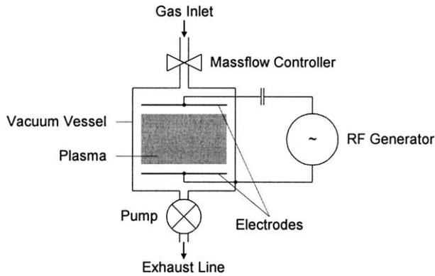
Fig. 1. Capacitively coupled RF-powered plasma.
