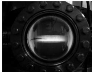
Fig. 5. Langmuir probe in Argon plasma
